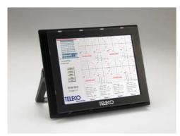
SHM602 is an advanced integrated system for structural health monitoring (SHM) of buildings and civil structures based on the analysis of the response of these structures to environmental (traffic or wind action) or artificial excitations. Differently from traditional systems, based on expensive seismic analog transducers and
